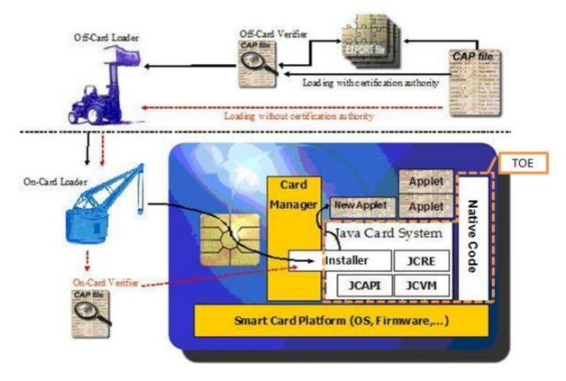
Figure 2: Java Card System and applet installation environment
