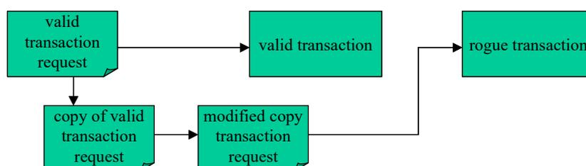
218 The picture shows a situation where the attacker copies a valid transaction request, modifies it and sends a second request using the same (or slightly modified) versions
