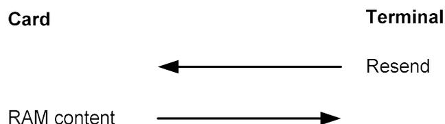
213 In this example, whether the TOE actually dumps the memory contents depends on the proper initialisation of I/O buffer pointer and length. The memory shown in the example might contain residual secret data, for example a recently calculated DES session key. Therefore this attack may allow an attacker to retrieve secret data from the TOE.
